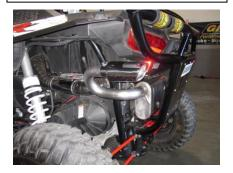
7. Once everything has been installed and tighten install your supplied Gibson tips. Slide the tips on to your desired look and tighten down. Check for 1" clearance and go have fun.
