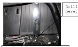
3. Next use a 4" drill bit to drill the hole for the tailpipe brackets. You will drill the lower threaded hole on the both driver and passenger side rear bed bracket. See above photo for location. Drill hole on both sides of the vehicle.
